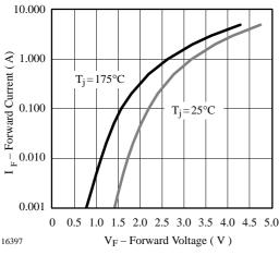
Figure 2. Forward Current vs. Forward Voltage
