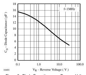
Figure 6. Diode Capacitance vs. Reverse Voltage
