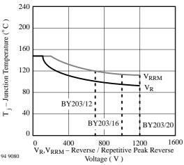
Figure 1. Junction Temperature vs. Reverse/Repetitive Peak Reverse Voltage
