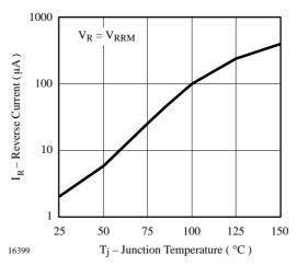
Figure 4. Reverse Current vs. Junction Temperature
