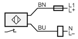
Note miniature fuse to IEC60127-2 sheet  $1 \le 2$  A fast acting
