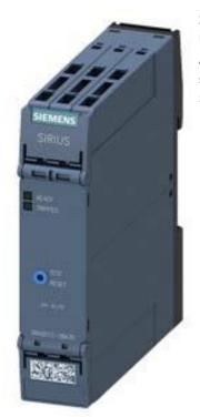
Thermistor motor prot. relay Standard evaluation unit 22.5 mm enclosure Spring-type terminals 2 CO contacts US = 24 V AC/DC Manual/Auto/Remote RESET with ATEX certification 2 LEDs (READY/TRIPPED) Galvanic separation Test/Reset button Open-circuit monitoring Short-circuit monitoring Non-volatile
