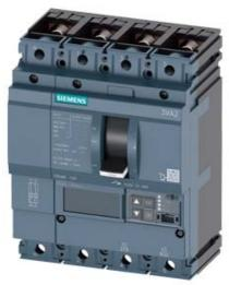
CIRCUIT BREAKER 3VA2 IEC FRAME 100 BREAKING CAPACITY CLASS H ICU=85KA @ 415 V 4POLE, LINE PROTECTION ETU850, LSI, IN=100A OVERLOAD PROTECTION IR=40A ...100A SHORT CIRCUIT PROTECTION ISD=0,6..10X IN, II=1,5..12X IN NEUTRAL PROTECTION ADJUSTABLE (OFF, UPTO 100%) BUSBAR CONNECTION
