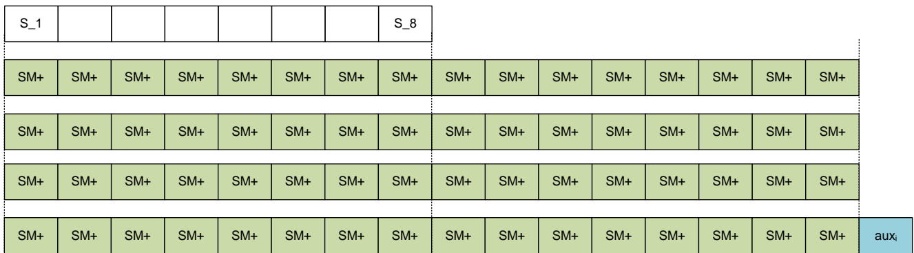
Figure 29: Sequencer Setup for Highest Update Rate on Bridge Sensor – aux i Executed after Eighth Measurement Cycle
