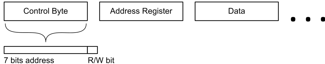
Figure 4 • High-Level Packet Structure
