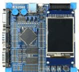
The Keil MCB2929 Evaluation Board introduces the NXP LPC2900 family of ARM9 processor-based devices, allowing you to create and test working programs for this advanced architecture. The MCB2929 has a wide range of interfaces making it a great starting point for your next ARM project.
