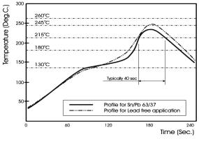
Infrared soldering profile
