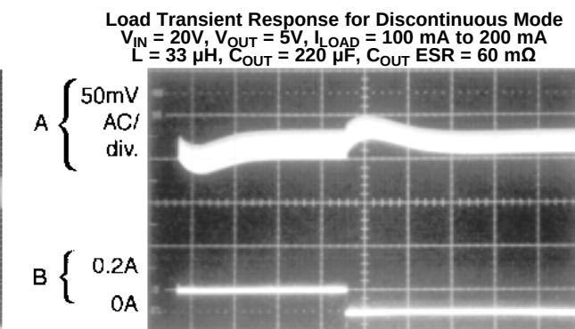
Figure 23. Horizontal Time Base: 2 \mu\text{s} /div.
