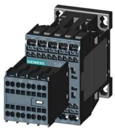
CONTACTOR RELAY, 6NO+2NC, AC 110V, 50/60 HZ, SZ S00, SPRING-LOADED TERMINAL, REMOVABLE AUX. SWITCH
