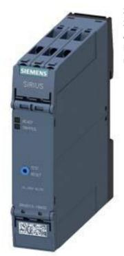
Thermistor motor prot. relay Standard evaluation unit 22.5 mm enclosure Screw terminals 2 CO contacts US = 24-240 V AC/DC Manual/Auto/Remote RESET with ATEX certification 2 LEDs (READY/TRIPPED)
