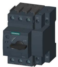
CIRCUIT-BREAKER SZ S00, FOR MOTOR PROTECTION, CLASS 10, W. OVERLOAD RELAY FUNCTION A-RELEASE 3.5...5A, N-RELEASE 65A, SCREW CONNECTION, STANDARD SW. CAPACITY
