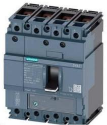
CIRCUIT BREAKER 3VA1 IEC FRAME 160 BREAKING CAPACITY CLASS H ICU=70KA @ 415 V 4-POLE, LINE PROTECTION TM220, ATFM, IN=63A OVERLOAD PROTECTION IR=44,1A ...63A SHORT CIRCUIT PROTECTION II=10 X IN NEUTRAL UNPROTECTED BUSBAR CONNECTION
