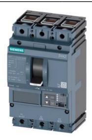
CIRCUIT BREAKER 3VA2 IEC FRAME 100 BREAKING CAPACITY CLASS H ICU=85KA @ 415 V 3POLE, LINE PROTECTION ETU860, LSIG, IN=25A OVERLOAD PROTECTION IR=10A ...25A SHORT CIRCUIT PROTECTION ISD=0,6..10X IN, II=1,5...12X IN NEUTRAL PROTECTION OPTIONAL WITH EXT. CT,UPTO 160% GROUNDFAULT, SWITCHABLE IG=0,2... 1 X IN, TG=0,050,8MS CABLE CONNECTION
