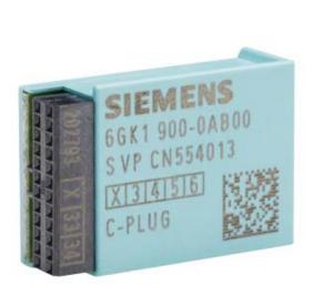
C-PLUG 256 (CP343-1 ADVANCED) REPLACEABLE MEDIUM FOR SIMPLE DEVICE EXCHANGE IN CASE OF FAILURE, FOR STORAGE OF CONFIGURATION OR USER DATA, 256MB, CAN BE USED IN CP343-1 ADVANCED
