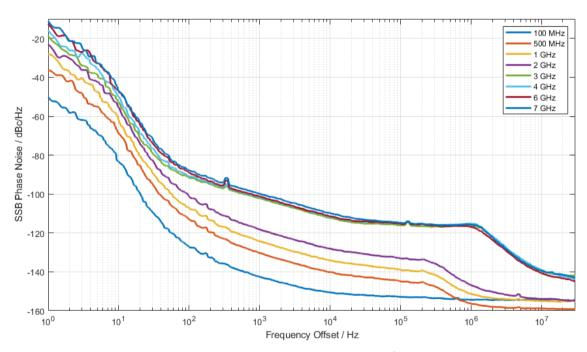
Measured SSB phase noise for different carrier frequencies, with R&S $^{\otimes}$ SMCVB-K709 option
