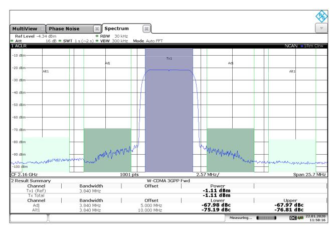
Measured ACPR for 3GPP test model 1, 64 DPCH
