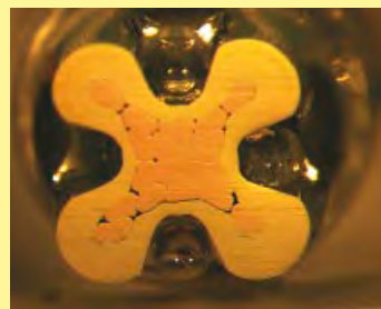
Crimp-cross section HARTING crimp profile
