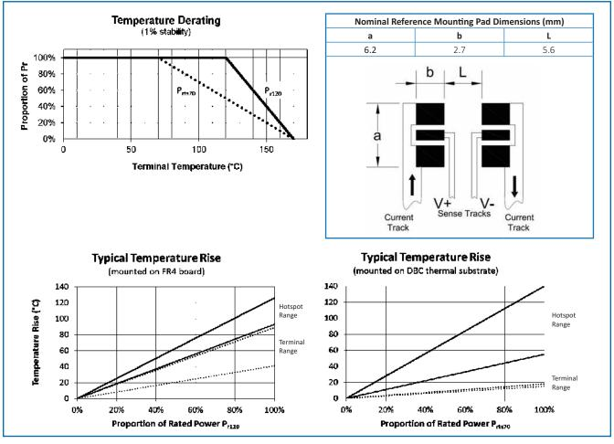
FR4 board details: 102x51mm, high Tg FR4 board with 70µm (2 ounce) inner and outer Cu planes or similar substrate, such that terminal temperature is maintained at ≤120°C.
