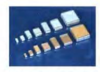
**Holy Stone** high voltage products are designed and manufactured to meet the general requirements of international standards. The product offering is well suited for commercial and industrial applications and includes NP0 (C0G) and X7R characteristics in sizes 0805 to 2225 and with working voltages from 1KV up to 5KV.
