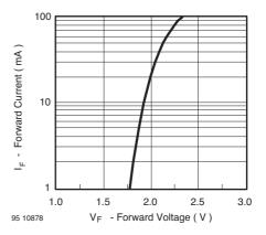
Figure 4. Forward Current vs. Forward Voltage
