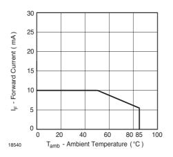
Figure 2. Forward Current vs. Ambient Temperature
