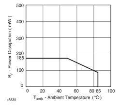
Figure 1. Power Dissipation vs. Ambient Temperature
