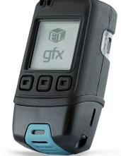
This stand-alone data logger measures and stores over 250,000 temperature and humidity readings over a -30 to  $+80^{\circ}$ C (-22 to  $+176^{\circ}$ F) and 0 to 100%RH range at a resolution of  $0.1^{\circ}$ C ( $0.1^{\circ}$ F) and 0.1%RH.
