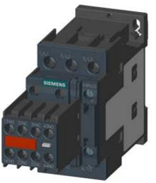
CONTACTOR, AC-3, 15KW/400V, 2NO+2NC, AC 230V 50/60HZ, 3-POLE, SZ S0 SCREW TERMINAL PERMANENT AUX. SWITCH FOR SUVA APPLICATIONS
