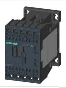
2NO+2NC CONTACTOR, AC3: 5.5KW AC 230V 50HZ 4-POLE, 2NO+2NC, SZ: S00, SPRING-LOADED TERMINAL
