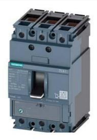
CIRCUIT BREAKER 3VA1 IEC FRAME 160 BREAKING CAPACITY CLASS H ICU=70KA @ 415 V 3-POLE, LINE PROTECTION TM220, ATFM, IN=20A OVERLOAD PROTECTION IR=14A ...20A SHORT CIRCUIT PROTECTION II=10 X IN CABLE CONNECTION
