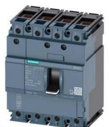
CIRCUIT BREAKER 3VA1 IEC FRAME 160 BREAKING CAPACITY CLASS H ICU=70KA @ 415 V 4-POLE, LINE PROTECTION TM210, FTFM, IN=63A OVERLOAD PROTECTION IR=63A FIXED SHORT CIRCUIT PROTECTION II=10 X IN NEUTRAL UNPROTECTED CABLE CONNECTION
