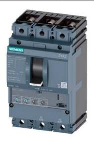
CIRCUIT BREAKER 3VA2 IEC FRAME 160 BREAKING CAPACITY CLASS M ICU=55KA @ 415 V 3POLE, LINE PROTECTION ETU330, LIG, IN=100A OVERLOAD PROTECTION IR=40A ...100A SHORT CIRCUIT PROTECTION II=1,5...12 X IN GROUNDFAULTPROTECTION IG=0,2... 1 X IN, TG=0,1/0,3MS BUSBAR CONNECTION
