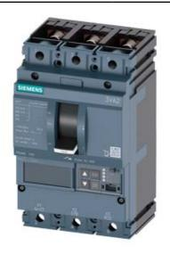
CIRCUIT BREAKER 3VA2 IEC FRAME 160 BREAKING CAPACITY CLASS H ICU=85KA @ 415 V 3POLE, LINE PROTECTION ETU560, LSIG, IN=160A OVERLOAD PROTECTION IR=64A ...160A SHORT CIRCUIT PROTECTION ISD=0,6..10X IN, II=1,5..10X IN NEUTRAL PROTECTION OPTIONAL WITH EXT. CT,UPTO 160% GROUNDFAULT, SWITCHABLE IG=0,2... 1 X IN, TG=0,050,8MS BUSBAR CONNECTION
