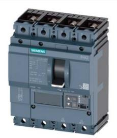
CIRCUIT BREAKER 3VA2 IEC FRAME 160 BREAKING CAPACITY CLASS H ICU=85KA @ 415 V 4POLE, LINE PROTECTION ETU550, LSI, IN=63A OVERLOAD PROTECTION IR=25A ...63A SHORT CIRCUIT PROTECTION ISD=0,6..10X IN, II=1,5..12X IN NEUTRAL PROTECTION ADJUSTABLE (OFF, UPTO 160%) BUSBAR CONNECTION
