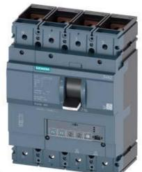
CIRCUIT BREAKER 3VA2 IEC FRAME 400 BREAKING CAPACITY CLASS H ICU=85KA @ 415 V 4-POLE, LINE PROTECTION ETU350, LSI, IN=250A OVERLOAD PROTECTION IR=100A ...250A SHORT CIRCUIT PROTECTION ISD=1,5... 10 X IR, II=12 X IN NEUTRAL PROTECTION ADJUSTABLE(OFF,50%,100%) BUSBAR CONNECTION
