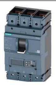
CIRCUIT BREAKER 3VA2 IEC FRAME 400 BREAKING CAPACITY CLASS H ICU=85KA @ 415 V 3-POLE, LINE PROTECTION ETU850, LSI, IN=250A OVERLOAD PROTECTION IR=100A ...250A SHORT CIRCUIT PROTECTION ISD=0,6..10X IN, II=1,5..12X IN NEUTRAL PROTECTION OPTIONAL WITH EXT. CT;UPTO 160% BUSBAR CONNECTION
