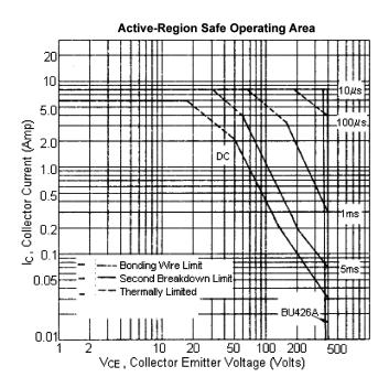
There are two limitations on the power handling ability of a transistor: average junction temperature and second breakdown safe operating area curves indicate  $\rm I_C\text{-}V_{CE}$  limits of the transistor that must be observed for reliable operation i.e., the transistor must not be subjected to greater dissipation than the curves indicate.
