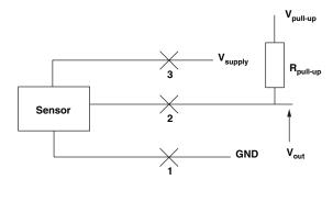
$V_{pull-up}$  can be independent to  $V_{supply}$
