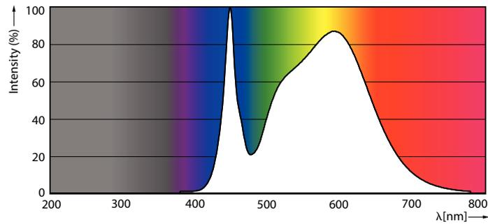
Spectral Power Distribution Colour - MAS LEDtube 900mm HO 18.5W 840 T5
