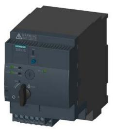
SIRIUS, COMPACT STARTER, REVERSING STARTER 400 V, 110 ... 240 V AC/DC, 50 ... 60 HZ, 8 ... 32 A, IP20, MAIN CIRCUIT CONNECTION: PLUG-IN, W/O TERMINALS, AUXILIARY CIRCUIT CONNECTION: SCREW TERMINAL
