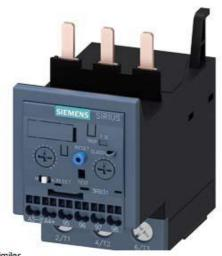
OVERLOAD RELAY 12.5...50 A FOR MOTOR PROTECTION SIZE S2, CLASS 5E...30E FOR MOUNTING ONTO CONTACTORS MAIN CIRCUIT: SCREW TERMINAL AUX. CIRCUIT: SPRING-TYPE TERM. MANUAL-AUTOMATIC-RESET INT. GROUND FAULT DETECTION
