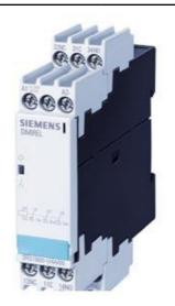
COUPLING RELAY IM INDUSTRY-STANDARD ENCLOSURE 3 CHANGEOVER CONTACTS COMBIVOLTAGE 24 V AND 220 V TO 240 V AC/DC SCREW TERMINALS
