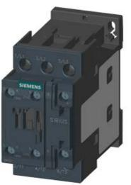
CONTACTOR, AC-3, 18.5KW/400V, 1NO+1NC, AC 400V 50HZ, 3-POLE, SZ S0 SCREW TERMINAL
