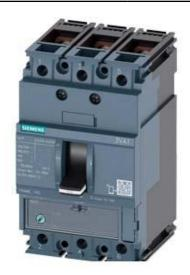
CIRCUIT BREAKER 3VA1 IEC FRAME 160 BREAKING CAPACITY CLASS S ICU=36KA @ 415 V 3-POLE, LINE PROTECTION TM220, ATFM, IN=80A OVERLOAD PROTECTION IR=56A ...80A SHORT CIRCUIT PROTECTION II=10 X IN BUSBAR CONNECTION
