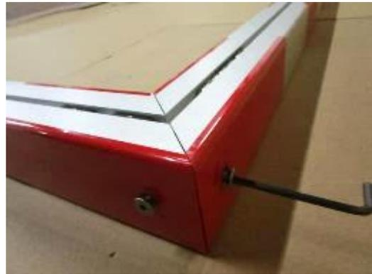
Advice: Due to production tolerances of the aluminium cast corner joints problems during adjustment of corners may possibly occur. Then shorten the stamps in the uprights with a flat file.
