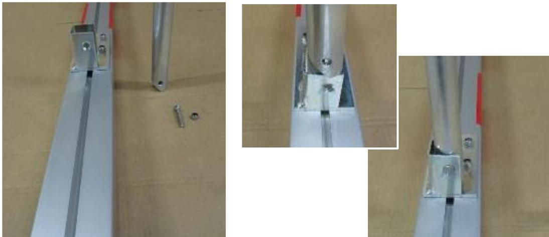
h) Assembly of ring nut: Stick from the inside ring nuts M8 x 50 through lateral and upper net hoop holes and fix them with cap nuts M8, DIN 986 (see bottom picture).
