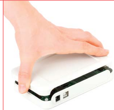
Figure 8-3: Place cover casing plastic and wind screws into outer screw holes to fix it with bottom plastics casing
