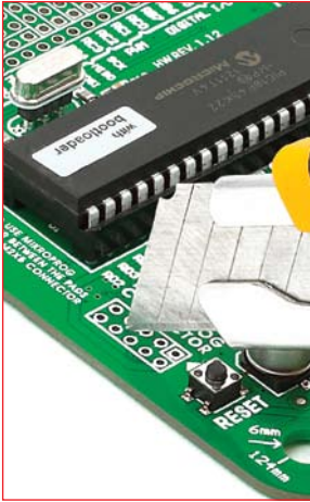
Figure 3-2: cutting copper between pads
