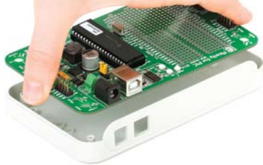
Figure 8-1: Place the board into the bottom part of the casing. Make sure that connectors are aligned with square openings
