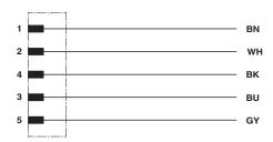
Contact assignment of the M12 connector
