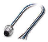
Sensor/actuator flush-type plug, 5-pos., M12-SPEEDCON, A-coded, front/screw mounting with M16 thread, with 0.5 m TPE litz wire,  $5 \times 0.34 \text{ mm}^2$
