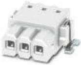
PCB headers, nominal current: 6 A, rated voltage (III/2): 160 V, number of positions: 4, pitch: 2.5 mm, color: white, contact surface: Tin, mounting: SMD soldering, Article with anti-rotation pin
