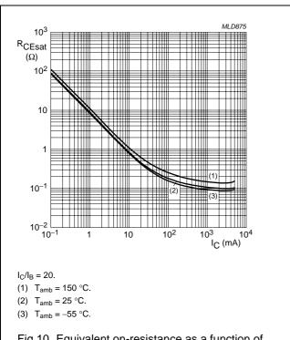
Fig.10 Equivalent on-resistance as a function of collector current; typical values.
