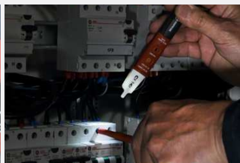
Built-in worklight (NCV-1030-EUR Voltfix, NCV-1040-EUR MAGNO-VOLTfix)
