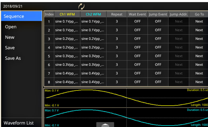
Advanced mode lets you build complex waveform sequences with flexible step controls
