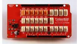
The one labeled IO (D13, D12, D8, D7, D4, D2) are Input
