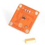
potentiometer, a signal amplifier, the standard TinkerKit 3pin connector, a green LED that signals that the module is correctly powered and a yellow LED whose brightness changes according to the position of the potentiometer.
