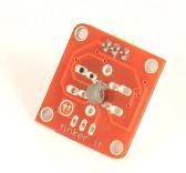
A **Hall sensor** creates a voltage related to the magnetic field around the sensor. This can be used to detect distance from a nearby magnet. Hall sensors can also be used to detect the magnetic field induced in a wire or coil.
