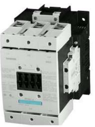
CONTACTOR, 55KW/400V/AC-3, AC(40...60HZ)/DC OPERATION UC 240...277V AUX. CONTACTS 2NO+2NC, 3-POLE, SIZE S6 WITH BOX TERMINALS CONVENTIONAL OPERATING MECHAN. SCREW TERMINAL
