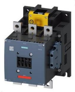
Contactor AC3: 132kW / 400 V 3-pole Size S10 Coil AC 50/60Hz and DC 96...127 V x (0,8...1,1) auxiliary contacts: 2 NO + 2 NC permanently mounted (SUVA) Main: busbar connections coil and auxilliary: screw terminal
