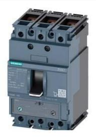
CIRCUIT BREAKER 3VA1 IEC FRAME 160 BREAKING CAPACITY CLASS S ICU=36KA @ 415 V 3-POLE, LINE PROTECTION TM240, ATAM, IN=63A OVERLOAD PROTECTION IR=44,1A ...63A SHORT CIRCUIT PROTECTION II=5...10 X IN BUSBAR CONNECTION
