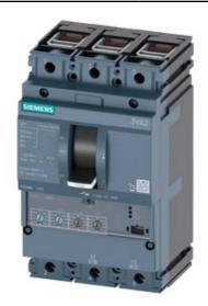
CIRCUIT BREAKER 3VA2 IEC FRAME 100 BREAKING CAPACITY CLASS C ICU=110KA @ 415 V 3POLE, LINE PROTECTION ETU330, LIG, IN=100A OVERLOAD PROTECTION IR=40A ...100A SHORT CIRCUIT PROTECTION II=1,5...12 X IN GROUNDFAULTPROTECTION IG=0,2... 1 X IN, TG=0,1/0,3MS CABLE CONNECTION
